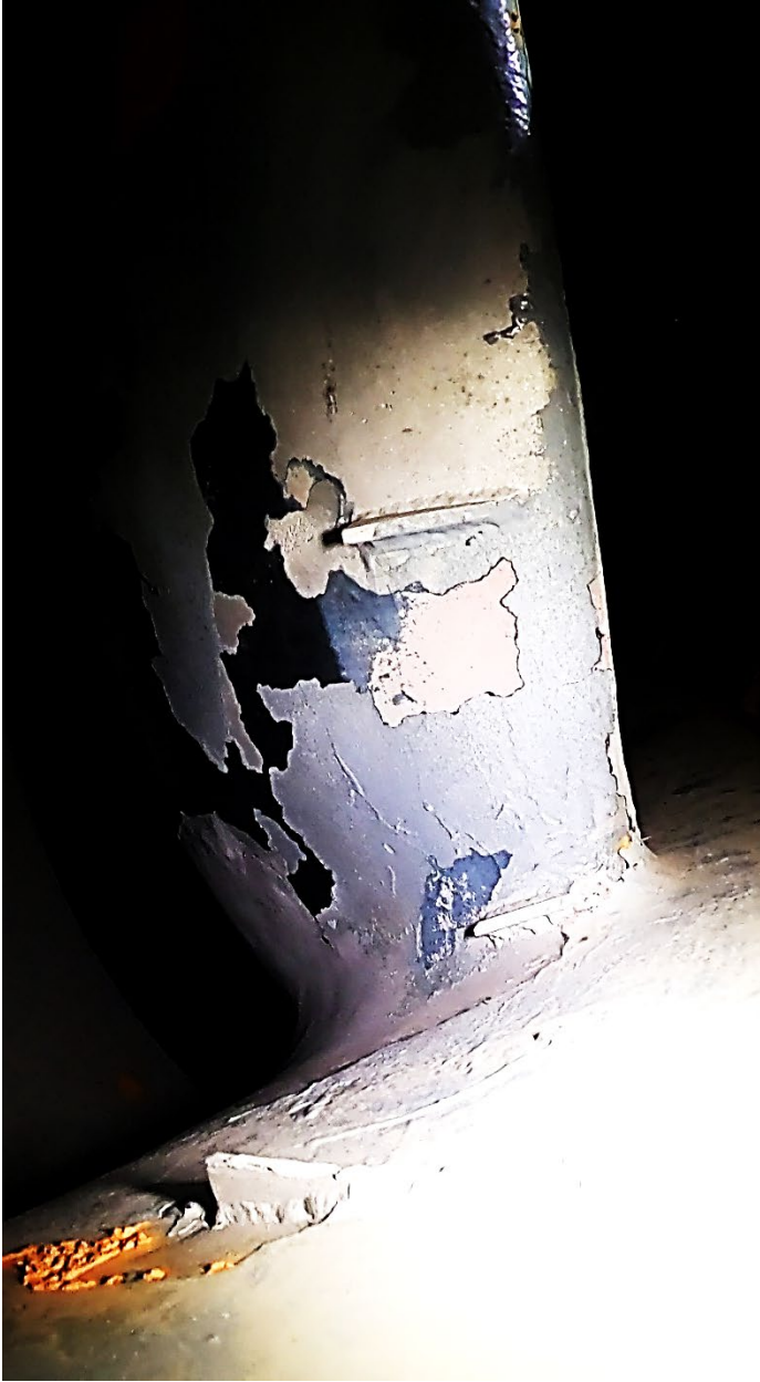
Figure 14.—Close-up of Blade 7 after 1,000 hours of operation. The PE2 failed by cavitation and delamination on leading edge.
