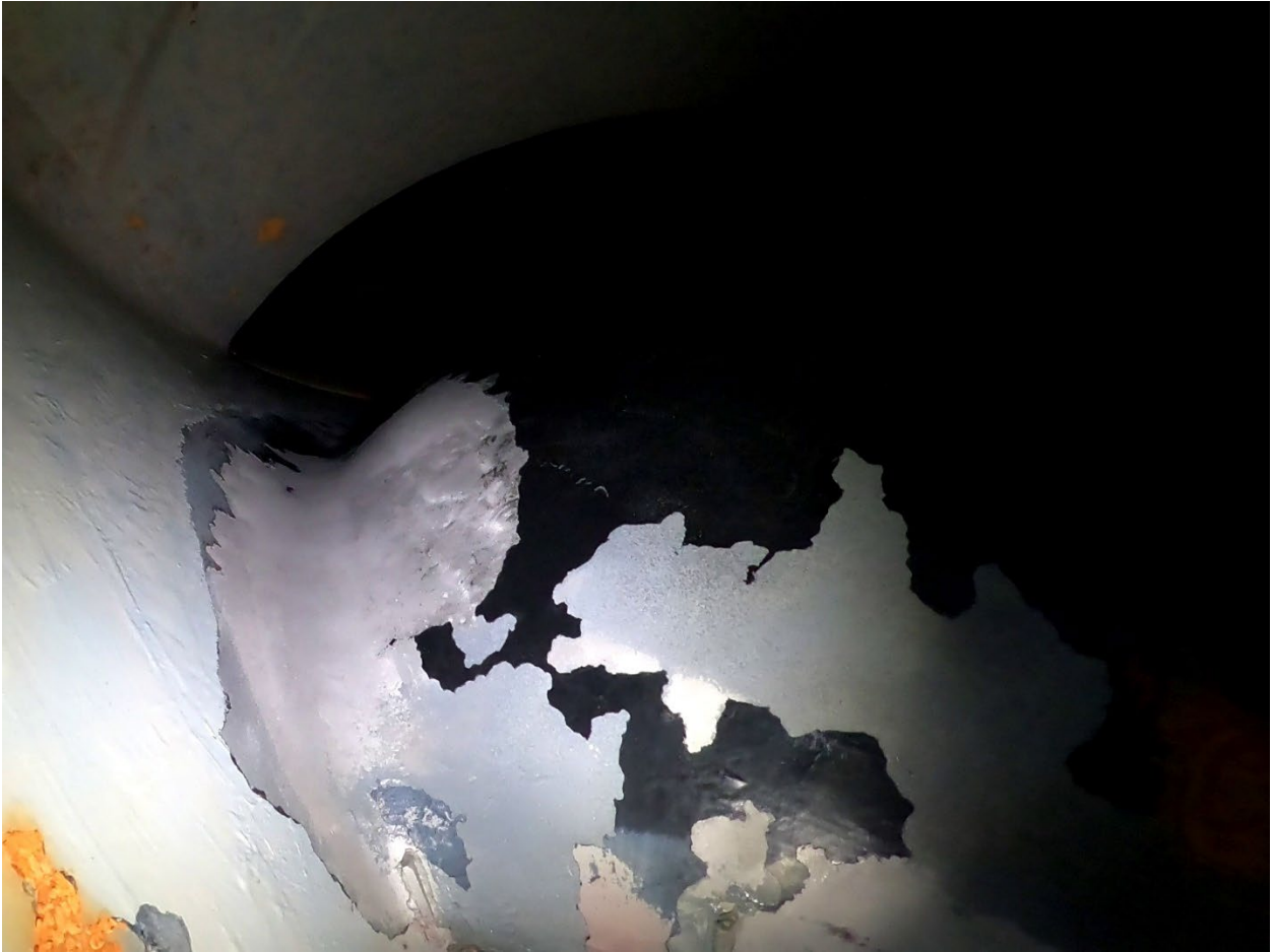
Figure 15.—Close-up of Blade 7 after 1,000 hours of operation. The PE2 failed by cavitation and delamination.
