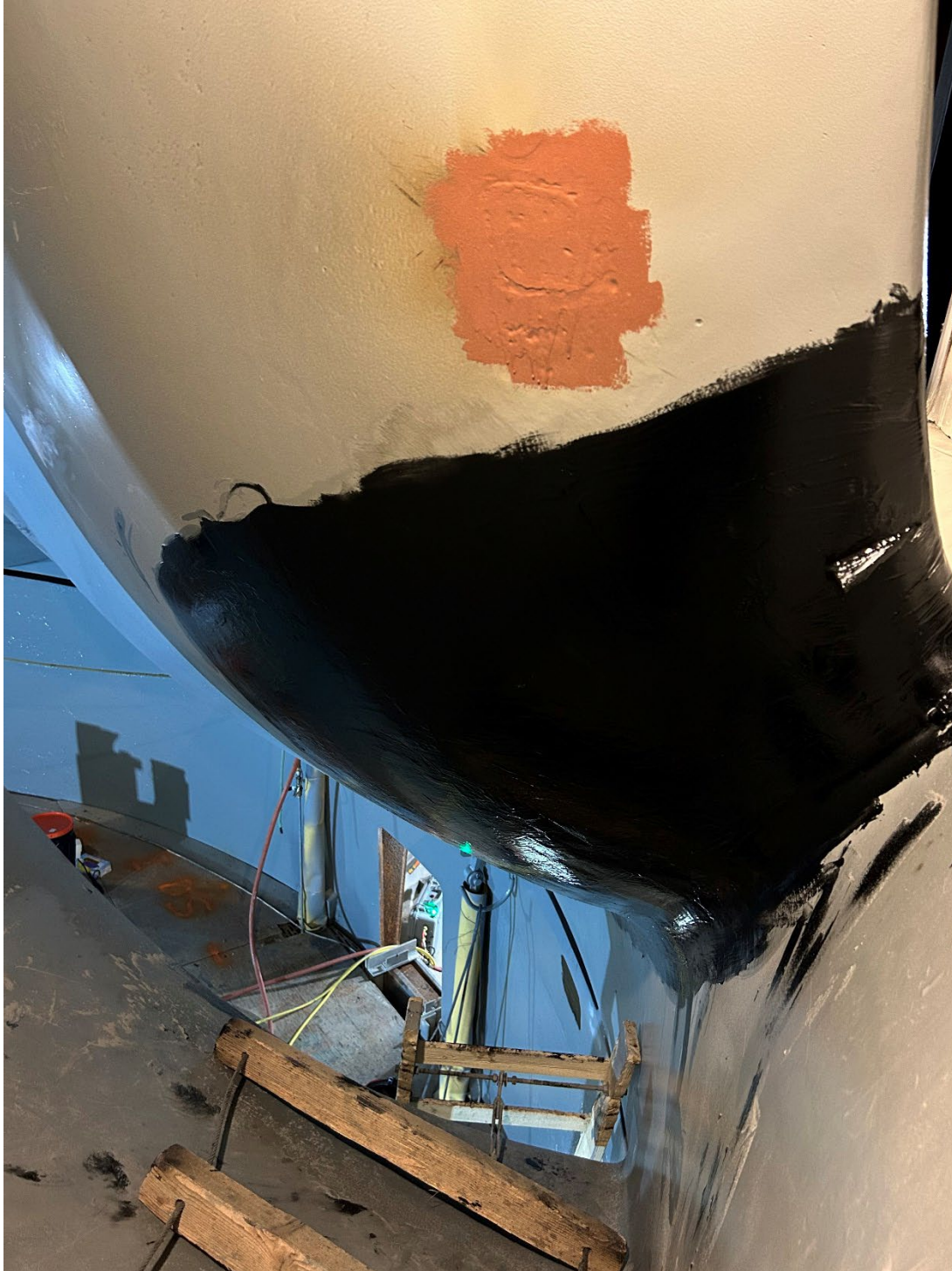
Figure 11.—The cavitation zone of Blade 8 shown coated with solvent-borne epoxy and PE2 before exposure.
