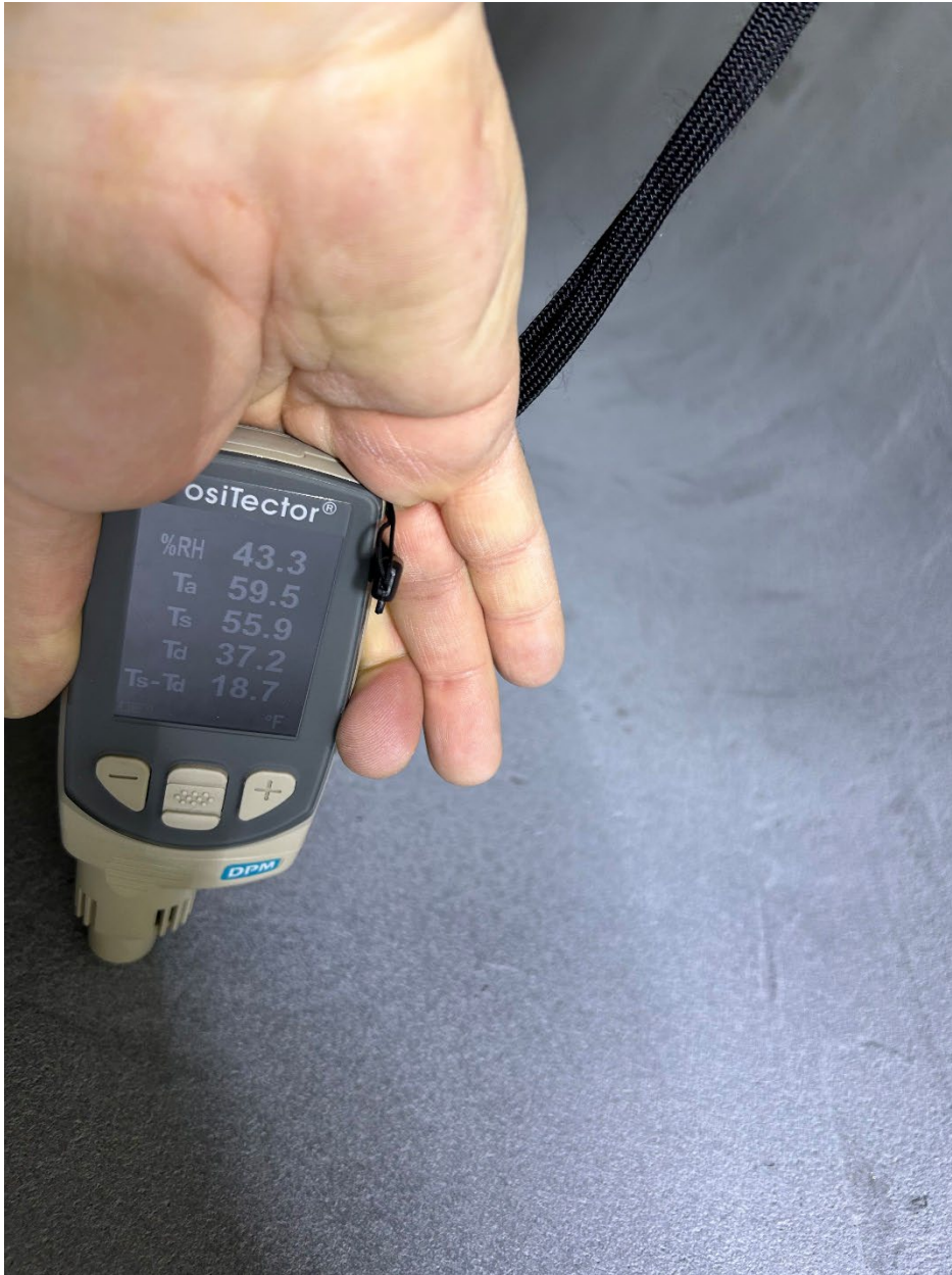
Figure 3.—Measurement of environmental conditions on Blade 13 prior to the application of adhesive.
